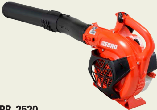
PB-2520 Engine displacement: 25.4cm³ // Output: 0.9kW / 1.2ps // Dry weight*2: 3.9kg // Blowing air force*3*5: 15.8N // Air volume*3*5: 768m³/h // Max. air speed*3*5: 76.2m/sec CE Posi-loc E
