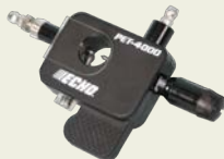
PET-4000 Ignition Checker Parts No. 897800-79931
